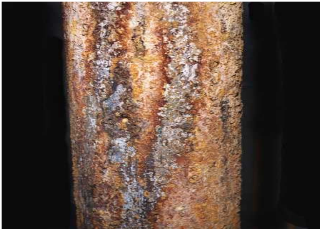
Fig.D1 General corrosion of external surface of pipework
