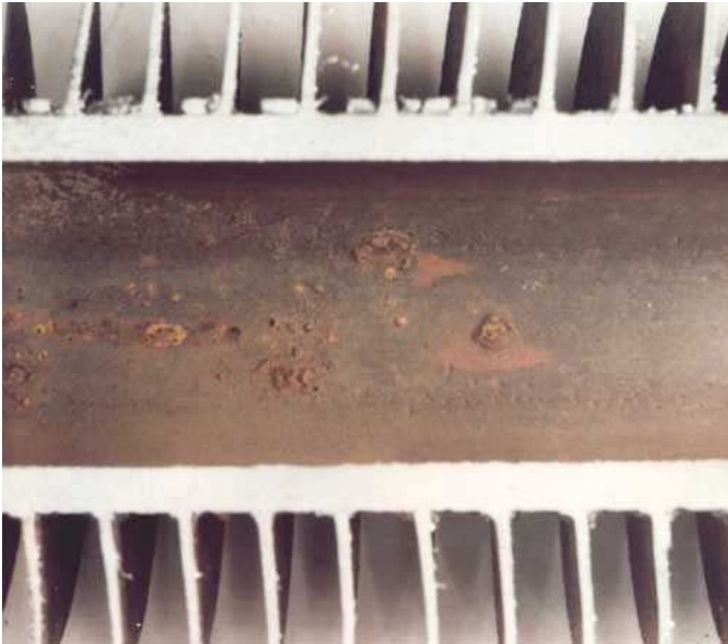
Fig.D2 Localised corrosion pitting of internal surface of finned pipework
