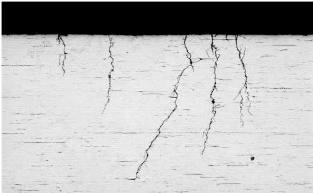
Fig.D7 Microscopic detail of stress corrosion cracking
