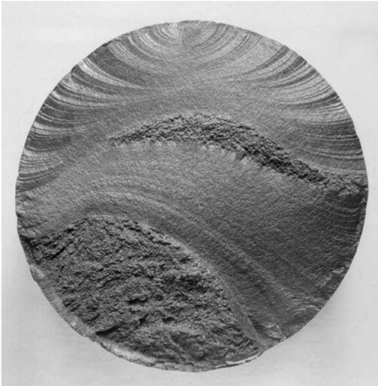
Fig.D5 Fatigue damage of shaft
