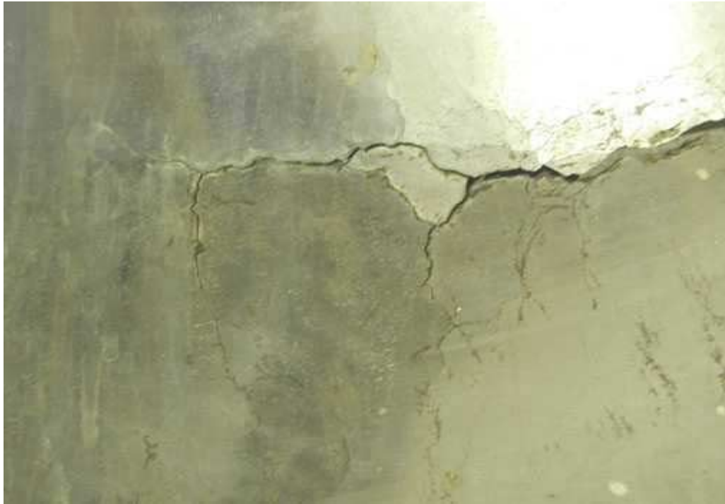
Fig.D6 Stress corrosion cracking in vessel shell
